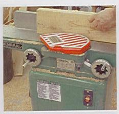
**STEP 24** • Next, press the flat face against the jointer fence and mill one edge at 90° to the prepared face.
