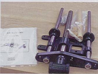
STEP 30 ■ My front vise is a single-screw model made by Veritas Tools, available from Lee Valley Tools. I followed the installation instructions and added two 1½\*-thick wood jaws.
