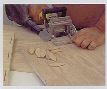
STEP 11 I used three #20 biscuits and glue to attach the carcass sides E to the bottom and top boards F. Dowels or screws and glue can also be used.
