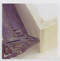
STEP 17 = Join the drawer box sides to the back and front boards using glue and 1" brad nails. The nails will hold the joint until the glue dries. Glue and nail the bottom boards to the drawer box frames.
