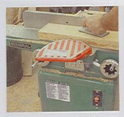
STEP 23 = To prepare rough boards for joining, flatten one face on a jointer.
