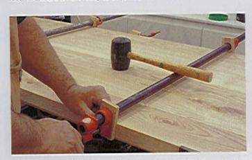
STEP 27 ■ Join the boards with clamps on the top and bottom face as shown. This over-and-under technique will help to ensure that your top will set up flat. Tighten the clamps until you see just a little of the glue squeeze out. Clamps set too tight will squeeze out a lot of glue, starving the joint and possibly making it fail.
