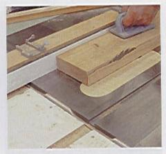
STEP 25 Cut the remaining rough edge parallel to the jointed edge, and at 90° to the prepared face, on a table saw. Hold the jointed edge of the board tight to the saw fence and the prepared face flat on the saw table.
