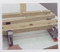
STEP 3 Glue two horizontal supports A together, forming a board with three 1"-square through-mortises. The eight supports will make four horizontal support members. Use dowels, biscuits or simply edge-glue the pieces to each other.
