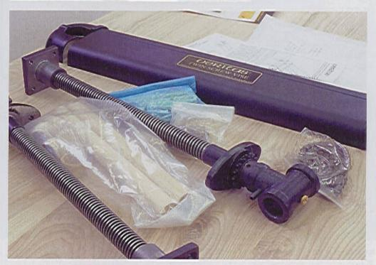
**STEP 31** The end vise I used is also made by Veritas and is a twin-screw model. When using large end vises on this bench, be sure the moving mechanics of the vise clear the bench supports. I used 7½"-high wood jaws, centering the screws 3" up from the bottom edge of the boards, so both screws would clear the upper horizontal supports.
