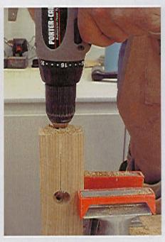
STEP 8 = Cut the two stretcher boards D to the size indicated in the materials list. Drill a 1"-diameter through-hole, centered 4" from each end on both stretchers. Then drill the ends of both boards using a 3/s"-diameter bit. The holes are located on the center of each end and are drilled 4" deep to meet the 1"-diameter through-holes.
