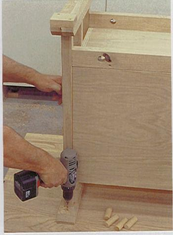
STEP 28 = Complete the top by scraping off the excess glue and sanding smooth. Trim to the required 30"-wide by 72"-long size. Turn the top facedown on the floor. Set the leg and carcass assembly upside down on the bottom face of the top so it's equally spaced side to side and front to back. Drill small pilot holes through the upper horizontal support and into the top. One hole at the end of each support is required.
