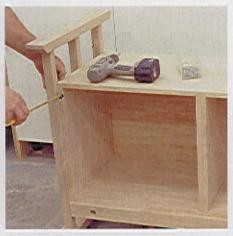
**STEP 14** Put the drawer carcass in the bench frame. Rest the bottom board on both stretchers, aligning the backboard with the outside face of the back stretcher. Use 1½° PB screws to secure the carcass to the bench frame. Do not use glue, so it can be removed if the bench must be moved.
