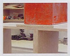
**STEP 12** Apply glue to both dadoes and place the dividers G into those dadoes. Use a heavy weight on top of the carcass until the adhesive sets and the dividers are fixed solidly n place.
