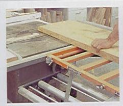
**STEP 1** = Rip and crosscut the eight horizontal supports A at  $1\frac{1}{2}$ "-square by 24"-long, and the six vertical supports B at  $1\frac{1}{2}$ "-square by  $33\frac{1}{2}$ "-long. A good crosscut blade on a table saw will be required to cut the  $1\frac{1}{2}$ "-thick material. A sliding table on your table saw, a radial-arm saw or power miter box can be used to crosscut the parts.
