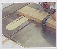
**STEP 2** The eight horizontal supports A each require three dadoes that are 1°-wide by ½°-deep. Two of the dadoes are located 3° from each end, and the third is located directly in the center. Dadoes can be cut on a table saw. If possible, gang four pieces together at one time and mark the pairs, this will ensure that sets are matched for joining.
