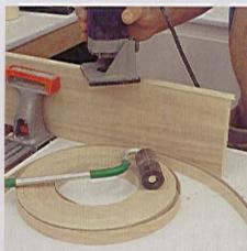
step 20 ■ The drawer faces Q, R and S are made using ¾<sub>6</sub>\*-thick veneer plywood. All four edges of each drawer face have wood veneer tape applied.
