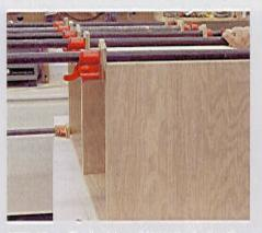
STEP 13 \* The backboard H is attached with #20 biscuits and glue. Clamp it in place until the adhesive sets up.
