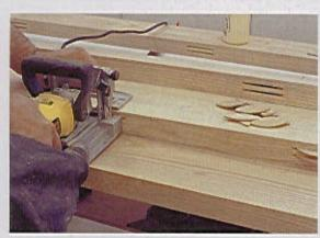
**STEP 22** ■ My benchtop T is constructed using six  $5\frac{1}{2}$ "-wide boards that are  $1\frac{1}{2}$ " thick. The boards are left longer than 72" and will be trimmed to size once the top is sanded. Thick boards can be joined with a double-biscuit technique that's shown in the photo.
