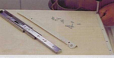
STEP 18 Attach drawer runners to each box. I am using  $\frac{1}{2}$ -extension glides, but full-extension glides (silver in the photo) can also be used if you require full access to the drawer. The full-extension models are two to three times more expensive than the  $\frac{1}{2}$ -extension type, but worth the extra cost if you need to fully access the drawer box.
