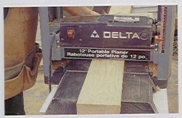
**STEP 26** Use a planer to dress the rough face parallel to the prepared face. The board is now ready to be joined to other boards.
