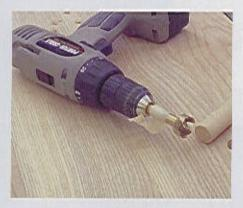
**STEP 29** • Drill 1\*-diameter holes, 1\* deep, in the bottom face of the top using the small drill holes from the previous step as a guide. Cut and install four  $2^{1/2}$ \*-long by 1\*-diameter dowels in the holes using glue.
