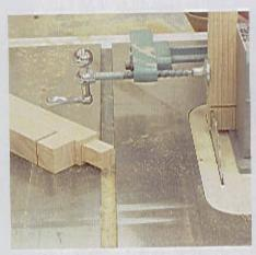
STEP 4 The six vertical supports B require a 1"-square by 1½"-long tenon centered on each end. These tenons can be cut on a table saw with a miter slide or, if you have one, a tenoning jig.
